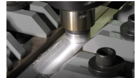
FSW (Friction Stir Welding 摩擦攪拌接合)
